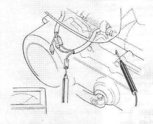
Check for continuity by attaching one test probe to yellow connector and the other to ground. Normal if there is continuity.
