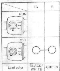
All wires are routed in headlight case. Check these switches when main switch is to be inspected.
