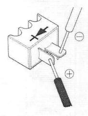
Normal if continuous only in arrow direction. Replace if continuity exists in reverse direction.
